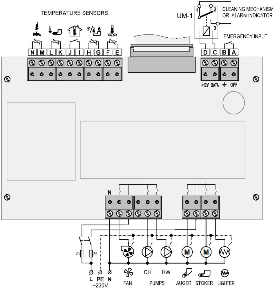
Figure 2. RK-2006LSP Controller connection diagram.
