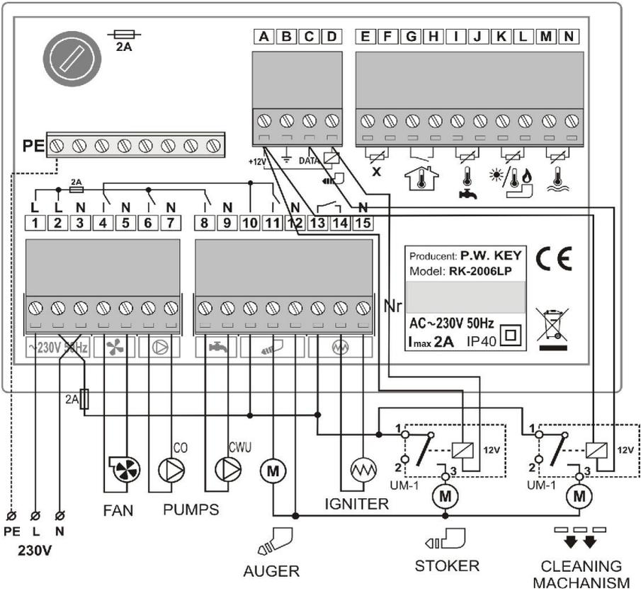
Figure 2. RK-2006LP Controller connection diagram.
