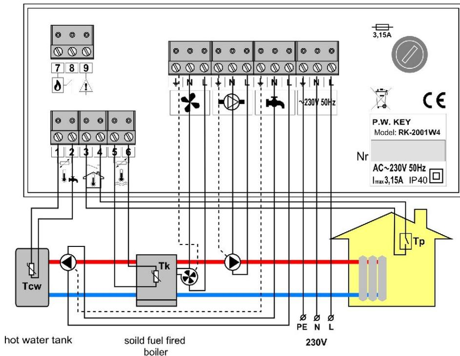
Picture 2. Schematics of connecting the RK-2001W4 unit.
